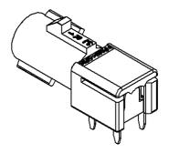
THE CONNECTOR MUST BE HOLD IN PLACE DURING THE SOLDERING OPERATION
